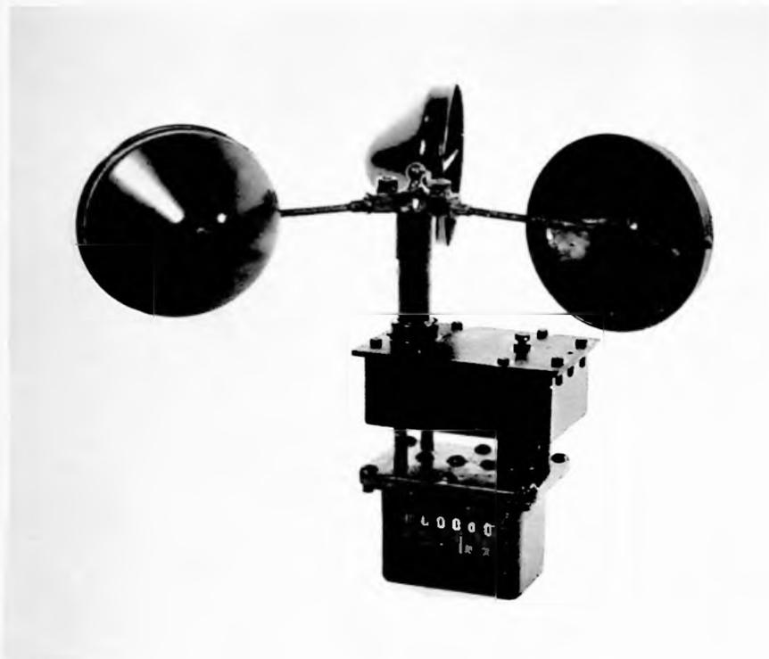
Fig. 27.—A modified cup-counter anemometer, Mk.2.
