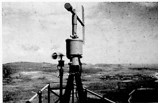
Fig. 5(c).—66-ft. mast at Anelog, showing wind-direction indicator and anemometer mountings.
