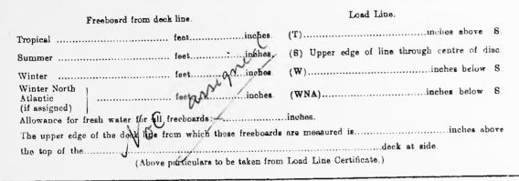
The Winter North Atlantic load line (if assigned) applies for Voyages across the North Atlantic, north of latitude 36\*N., during the winter months as defined in the Load Line Rules. The periods during which the other seasonal load lines apply in different parts of the world are as stated in the Load Line Rules.
