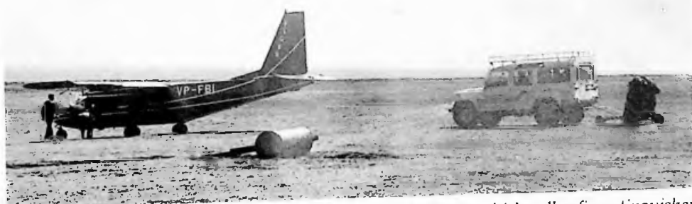
Emergency cover is provided on some grass strips by a Land-Rover which pulls a fire extinguisher
