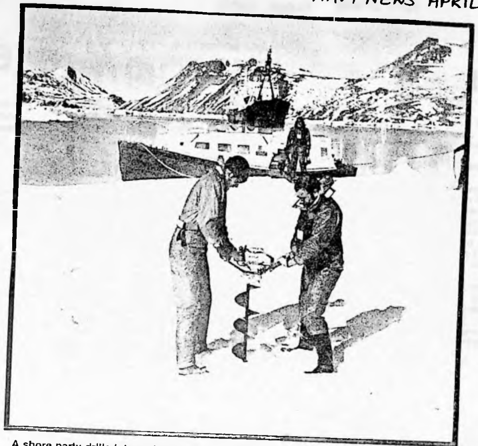
A shore party drills into an iceberg to provide HMS Endurance with a safe anchorage.
