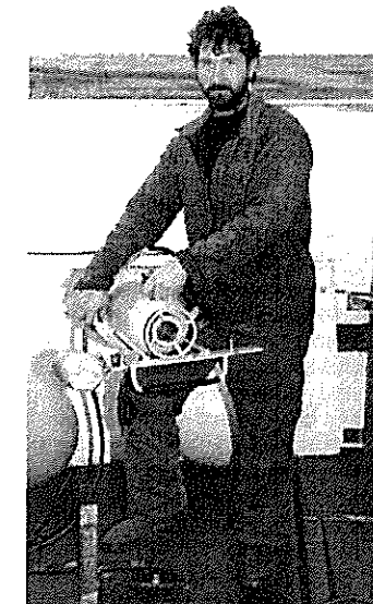
Paul Ellis holds part of the underwater camera unit. One of the two submarine lamps that it carries can be seen clamped to the crossbar. Extending from behind is the 'umbilical' hose through which are transmitted pictures from beneath the sea
