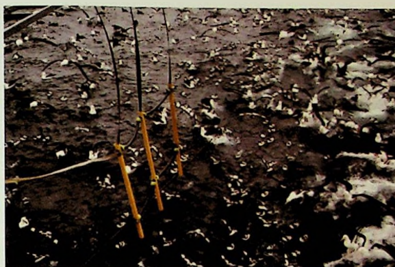
The Brady Baffler: as the fishing vessel pitches and rolls the ropes and cones swing and prevent birds from gathering in the area adjacent to the warp cable.
