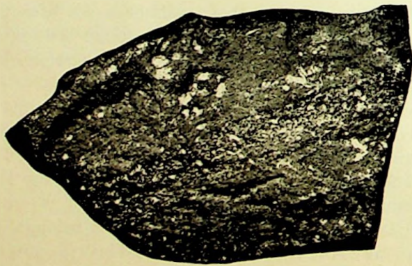
Fig. 11. Slate with a band of sandstone. Darwin Harbour. Nat. size. S. Bock phot.
